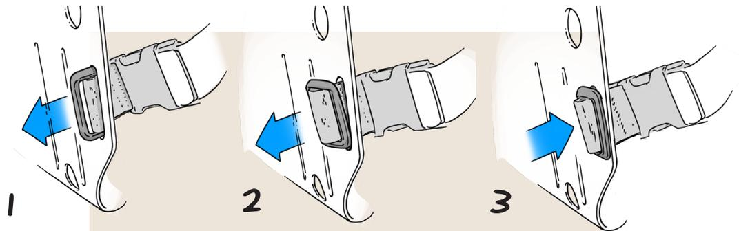
1-2\_ Insert the metal buckle sideways into the slot.
